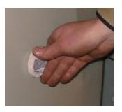
2. Daubrite® 1 VCI Emitter Packets: Protect multi-metal parts of enclosed space during storage and shipment, such as metals inside cabinets, boxes, bins, bags or envelopes. Do not open, simply place the Tyvek packet in the container with the parts and the embedded volatile corrosion inhibitor will create a chemical barrier on the surface of the metal.
