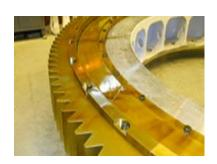
Nox-Rust® 5100: Ideal for general metal protection for indoor or outdoor storage environments for steel, compatible with non-ferrous metals. Use it with or without other barrier covers in domestic and export shipment and storage. It dries to a black, dry, firm film that can be handled after 3-6 hours and set up in 12-24 hours. Lasts 1-3 years in outdoor, unprotected storage; 3-5 years in protected outdoor storage. Easy to apply by spray, dip or brush. Remove with solvent / alkaline cleaner.
